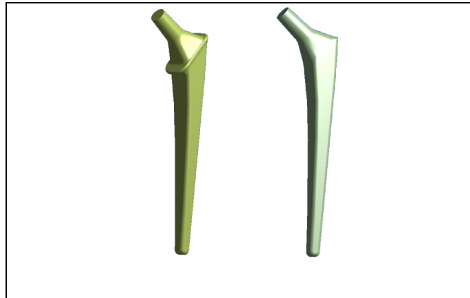
Fig. 2. CAD models of femoral stems with collar and without collar
